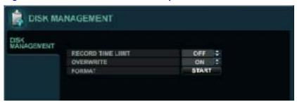
Highlight **DISK MANAGEMENT**, then press (4) to manage the internal hard drives.
