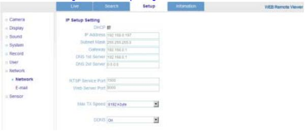
You can check the system's network information and selectable speed level. You cannot change IP settings. The network IP can be set only on the DVR. See *Configuring the Network Settings* on page 52 for more information.
