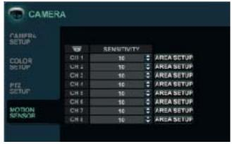
Use the to change the sensitivity level. The lowest level is 1, and the highest is 10. This setting determines the degree of motion required before recording is activated.
