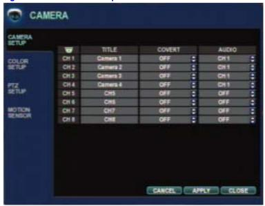
Figure 2-15 Camera Setup Window
