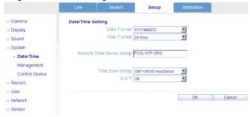
You can configure the date and time for the system, check system information, and configure the system ID, serial port protocol, and baud rate for the control device. See *Configuring System Settings* on page 46 for more information.
