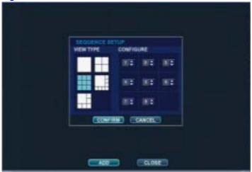
Select a screen display layout from the VIEW TYPE, select the channels for the layout from the CONFIGURE panel, then click CONFIRM.
