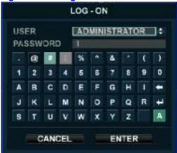
Enter the default password 1234 using the channel selection buttons, then press ENTER.
