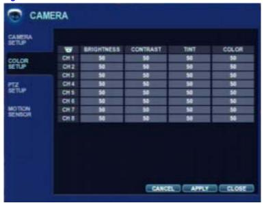
You can adjust the brightness, contrast, tint, and color for each channel. Select a channel and click on to select that channel for configuration. The selected channel displays full screen.
