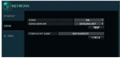
2. Turn **ON/OFF** the DDNS. When enabled, the DVR can be accessed through a Dynamic DNS server. This function is commonly used if your broadband connection does not have a static IP address.
