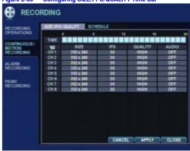
Figure 2-60 Configuring SIZE/FPS/QUALITY Time Bar
