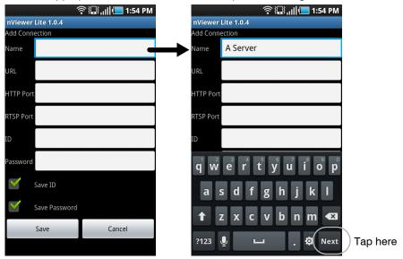
4. Continue through the remaining fields, entering the IP Address, HTTP and RTSP Port numbers, ID and Password for the HREP DVR (see <u>step 4</u> in <u>HREP DVR Network Configuration</u> for these values).
