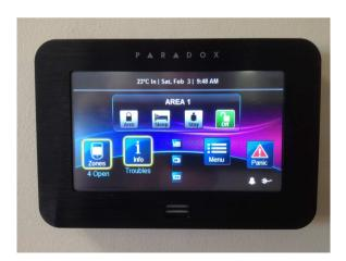
press 'DISARM' bottom right of the screen and put in a user code. If code does not work you can mute the codepad by pressing the 'Mute' button.
