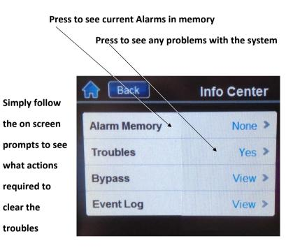
These 2 (alarm memory and troubles) are the most common used. Under troubles it is usually time and date (which can be fixed by pressing the line and setting the time and date.
