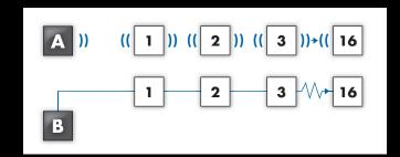
Each IntelliBox can control up to 16 Fog Cannons. Depending on the security class required, you either choose a wireless connection (A) or a cabled connection (B) - or a combination.
