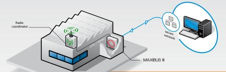
The radio coordinator is connected to MAXIBUS III. The integrated web server permits the configuration of the network and transmits all the alarm information.
